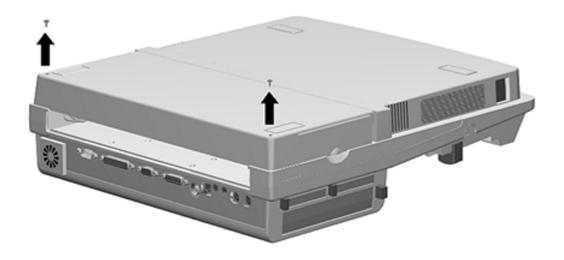
Figure 7-9. Removing the ISA Cover Screws
